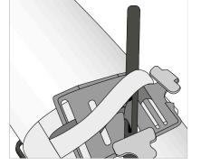
Lock the Tourniquet rod with one of the two fixation hooks
